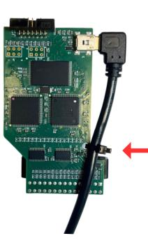
Example of ziptie used to secure the USB cable
